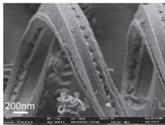
Fig. 21. SEM micrograph of CNC by the FE-SEM with a low acceleration voltage. Courtesy of Dr. Hamanaka at JFCC.
