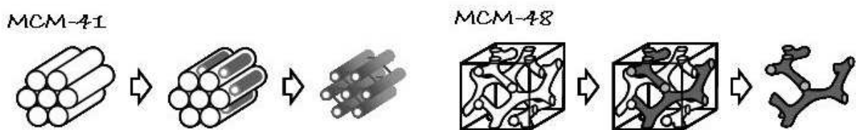
Fig. 1. Schematic illustration of the concept of M41S-template synthesis for ordered mesoporous carbons.
