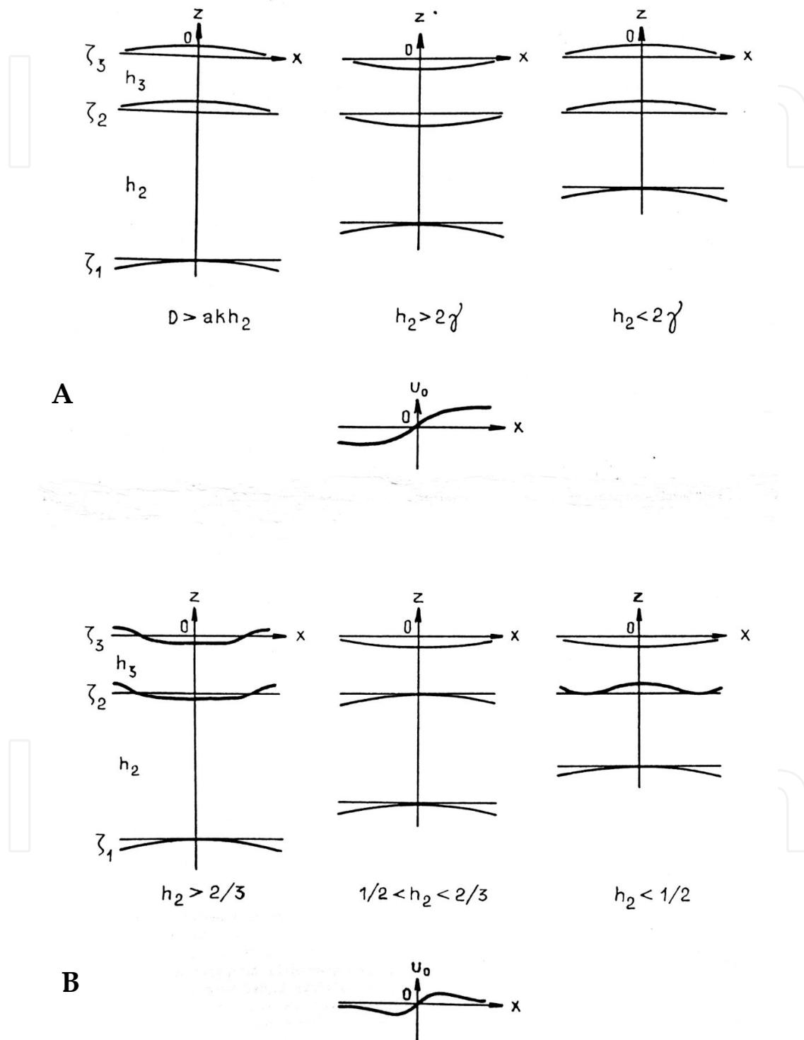
Fig. 3. Characteristic cross-sections of layers of earth crust and subjacent lithosphere above ascending mantle plume: a - without lateral limitations ( $U_0 = th kX$ ), b - with lateral limitations ( $U_0 = th kX / ch^2 kX$ ;  $D = 0$ )
