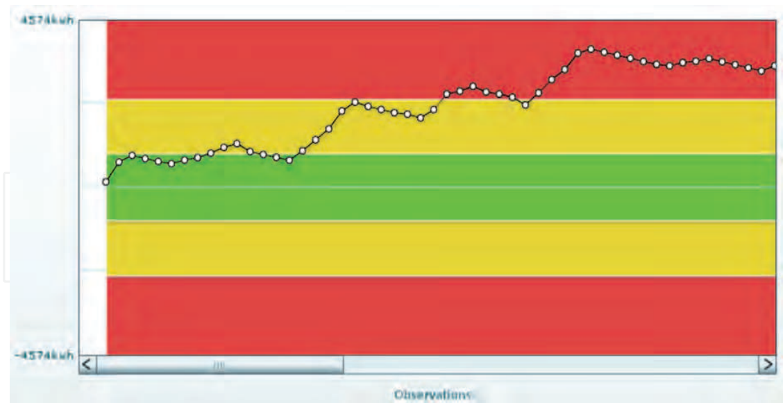
Fig. 10. CuSum of the hydraulic press energy consumption
