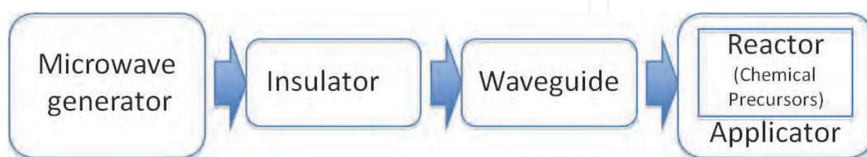
Fig. 9. Presentation of main elements of a classical microwave heating device
