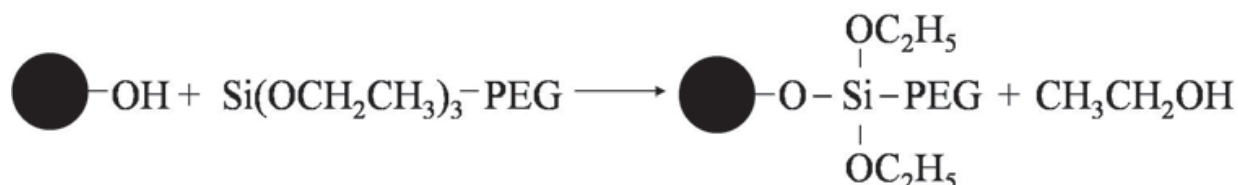
Fig. 6. Grafting reaction of functionalized PEG with magnetite nanoparticle (Zhang et al., 2002)
