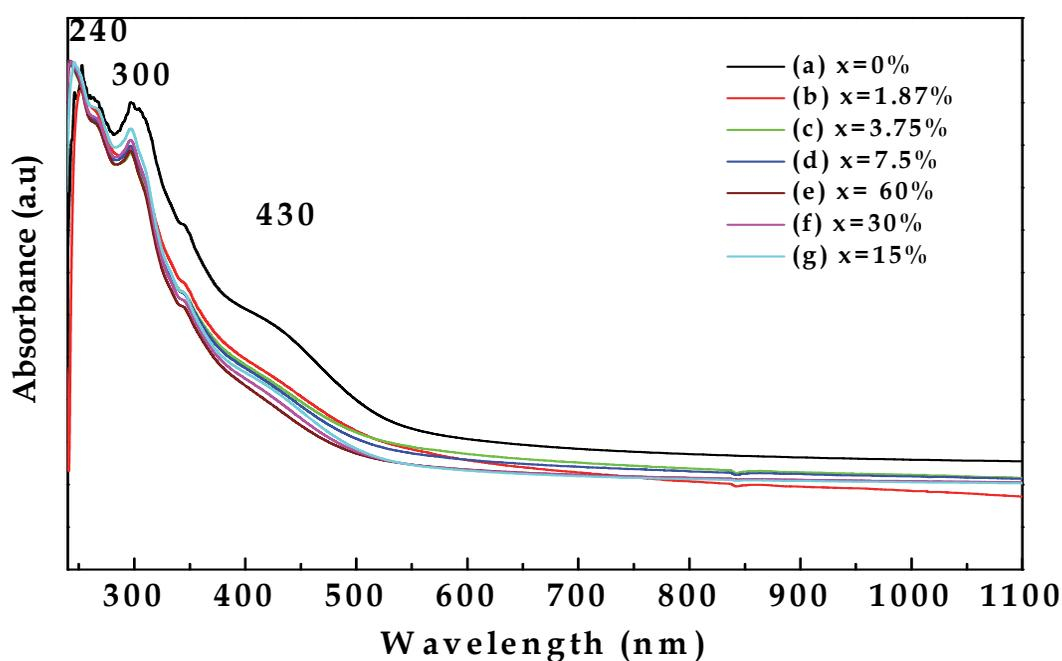
Fig. 18. Optical absorption at room temperature of pristine PVK-3HT (a) and those of PVK-3HT/SWNTs composites for different SWNTs weight concentrations (x): (a) Standard PVK-3HT, (b)  $x=1.87\%$ , (c)  $x=3.75\%$ , (d)  $x=7.5\%$ , (e)  $x=60\%$ , (f)  $x=30\%$ , and (g)  $x=15\%$ .
