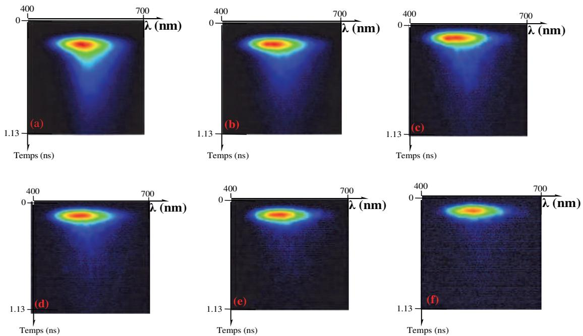
Fig. 20. Transient photoluminescence contour maps in false color of standard PVK-3HT (a) and those of PVK-3HT/SWNTs composites for different mass concentrations  $x$  of SWNT. (a) Standard PVK-3HT, (b)  $x=1.87\%$ , (c)  $x=7.5\%$ , (d)  $x=15\%$ , (e)  $x=30\%$ , (f)  $x=60\%$ .
