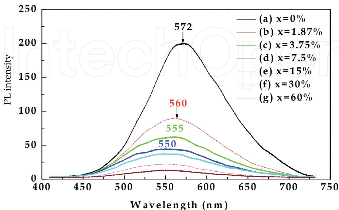
Fig. 19. Transient photoluminescence (TRPL) spectra in chloroform solution of pristine PVK-3HT (a) and those of PVK-3HT/SWNT composites for different SWNTs weight concentrations ( $x$ ) of SWNT: (b)  $x=1.87\%$ , (c)  $x=3.75\%$ , (d)  $x=7.5\%$ , (e)  $x=15\%$ , (f)  $x=30\%$ , (g)  $x=60\%$ .
