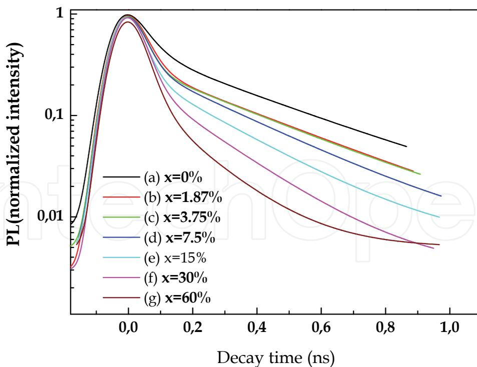
Fig. 21. Transient photoluminescence decays spectra of pristine PVK-3HT (a) and those of PVK-3HT/SWNT composites for different weight concentrations ( $x$ ): (b)  $x=1.87\%$ , (c)  $x=3.75\%$ , (d)  $x=7.5\%$ , (e)  $x=15\%$ , (f)  $x=30\%$  and (g)  $x=60\%$ .
