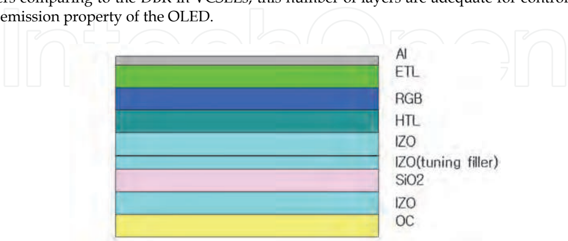
Fig. 4. The structure of strong cavity used for controlling the emission wavelength of white OLED.
