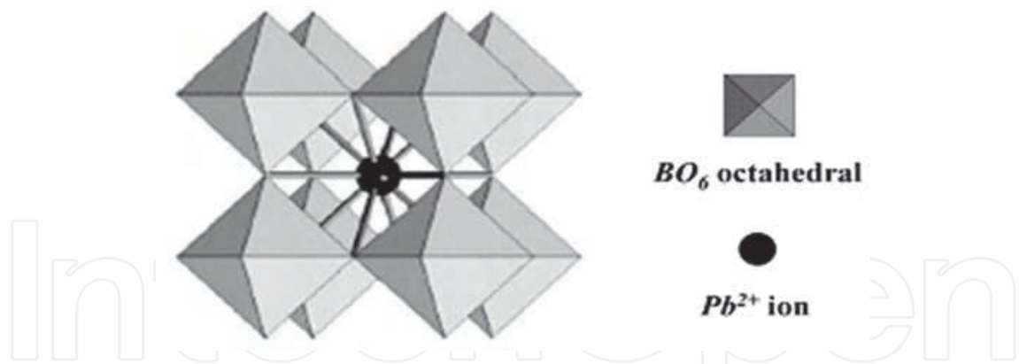
Fig. 10. Illustration of ideal ABO 3 -type perovskite structure, which can be described as a network of corner-linked octahedral.
