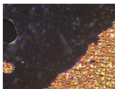
Fig. 14. Optical textures of (R)-III-(8,7) on a glass with a cover glass.
