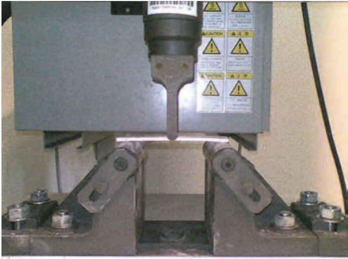
Fig. 10. Three point bending test setup
