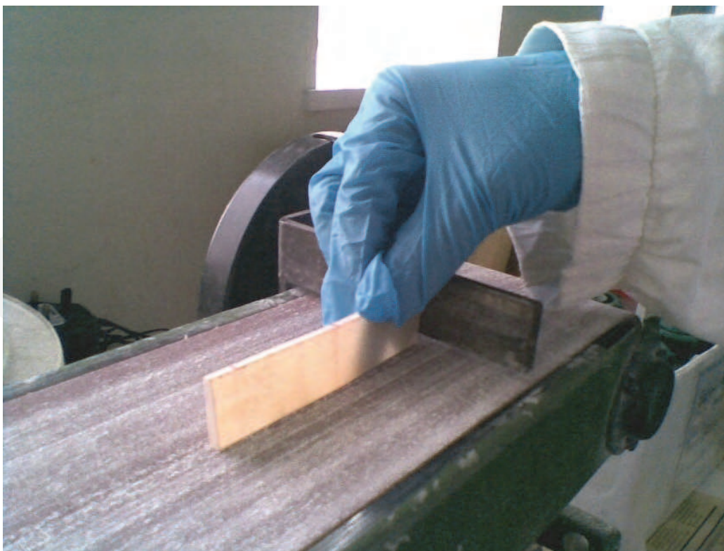
Fig. 9. Machining test specimen to size according to ASTM D790
