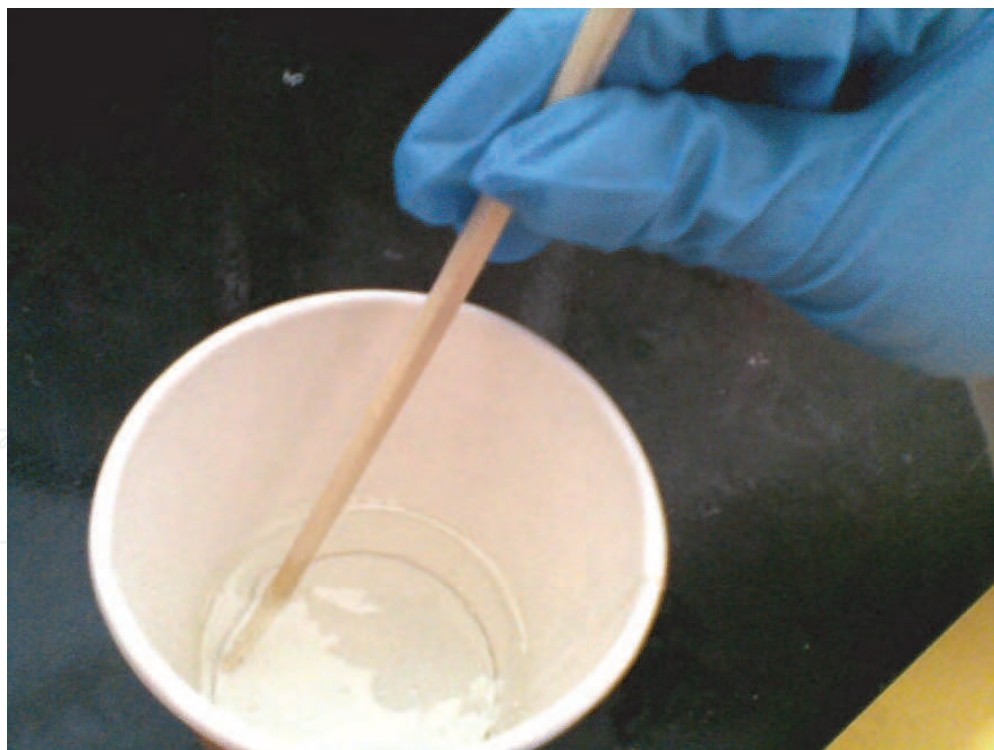
Fig. 3. Mixing of epoxy resin and hardener
