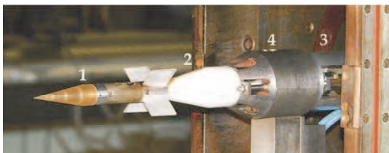
Fig. 8. Projectile model mounted on the free-pitching motion device in the wind tunnel
