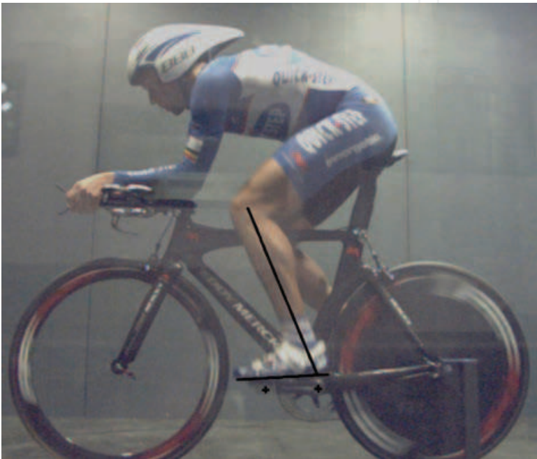
Fig. 10. Frame of the wind tunnel video-camera with drawn lines highlighting the pedaling angles
