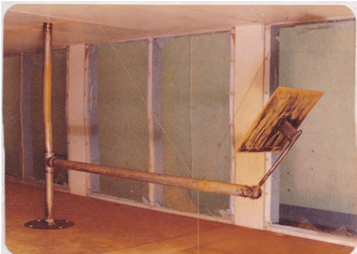
Fig. 7. Surface flow visualization setup
