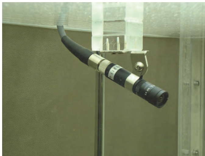
Fig. 9. Microcamera fixed on the ceiling of the tunnel at the downwind end.
