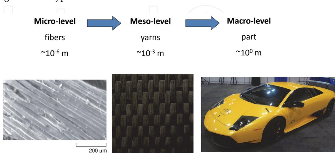
Fig. 1. 3 Hierarchical levels in woven fabrics
