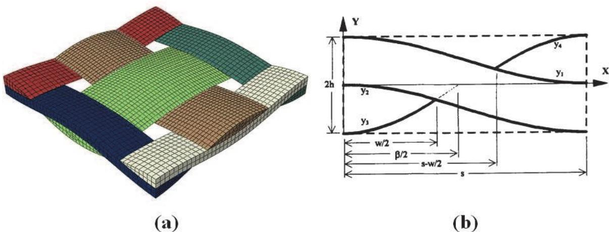
Fig. 3. (a) Schematic of the unit cell; (b) the yarn generating lines (Mcbride and Chen, 1997); For the current model,  $w = 2.11 \text{ mm}$ ,  $h = 0.5$  and  $S = 5.13$  are used. This means that the total length of the unit cell is  $2S = 0.26 \text{ mm}$ .
