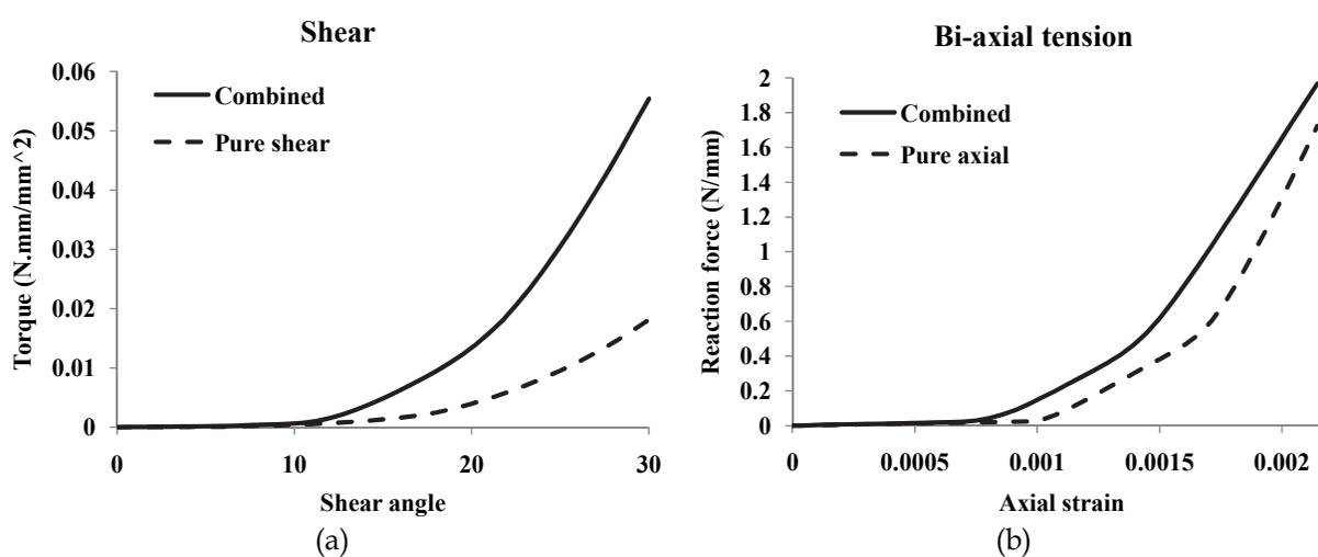
Fig. 8. The effect of combined loading on the reaction force and moment when compared to the individual (a) shear and (b) biaxial modes. The difference between curves in each graph indicates the presence of additional local deformation phenomena/ interactions between shear and axial modes under combined loading.
