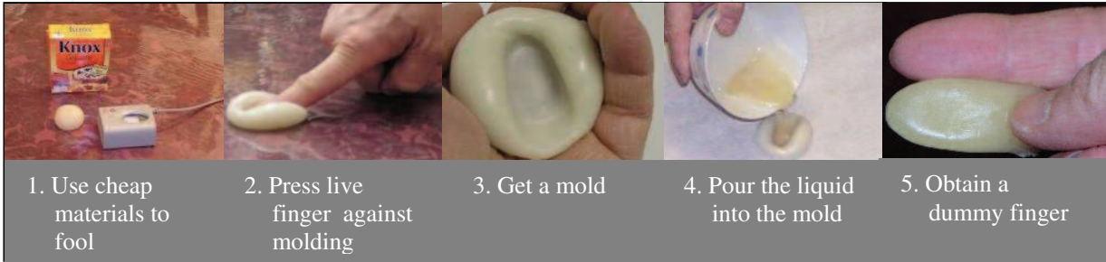
Fig. 17. Steps to make a dummy finger using a cheap kitchen powder
