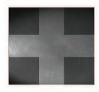
Fig. 24. Banded image of a real finger at 550nm wavelength with a band width of 300 pixels.
