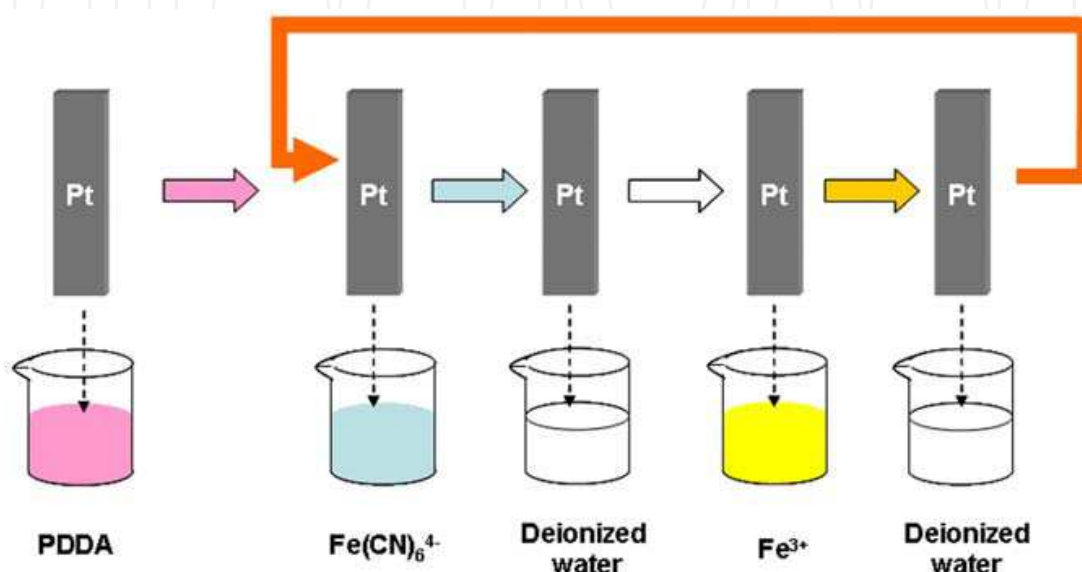
Scheme 1. Production of a PB-modified electrode using a self-assembly method.
