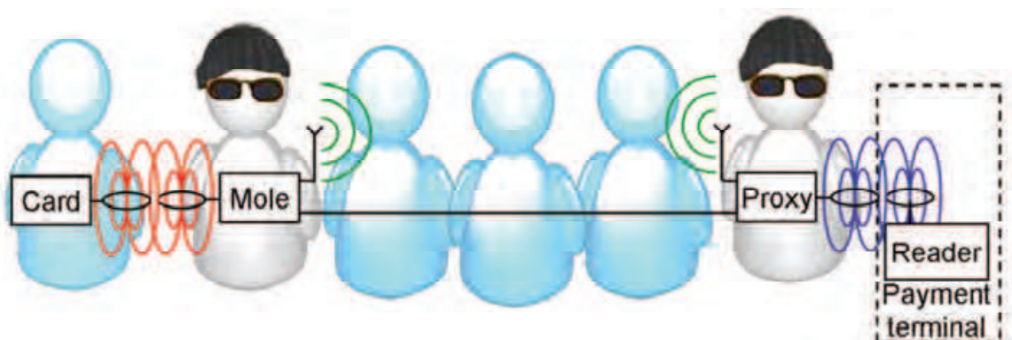
Fig. 12. Payment scenario: the relay attack setup
