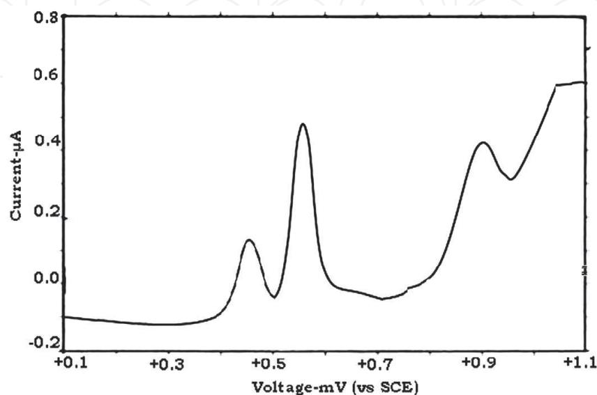
Fig. 8. Differential Pulse Voltammogram in 0.1M acetate buffer at pH  $4.5 \pm 0.1$ , obtained with a thin layer ds-DNA modified GCFE after being immersed in  $20 \mu\text{g/ml}$  epirubicin solution during 180 s, after applying a potential  $-0.60\text{V}$  during 60 s.
