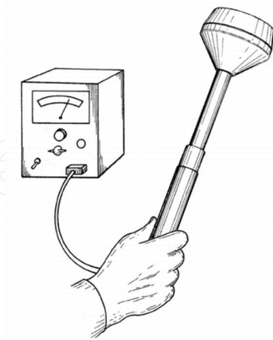
Fig. 10. Common Thermocouple Dosimeter. This design has been used for more than 60 years. The wideband thermocouple in probe's head makes it the best solution for Radiation dosimetry
