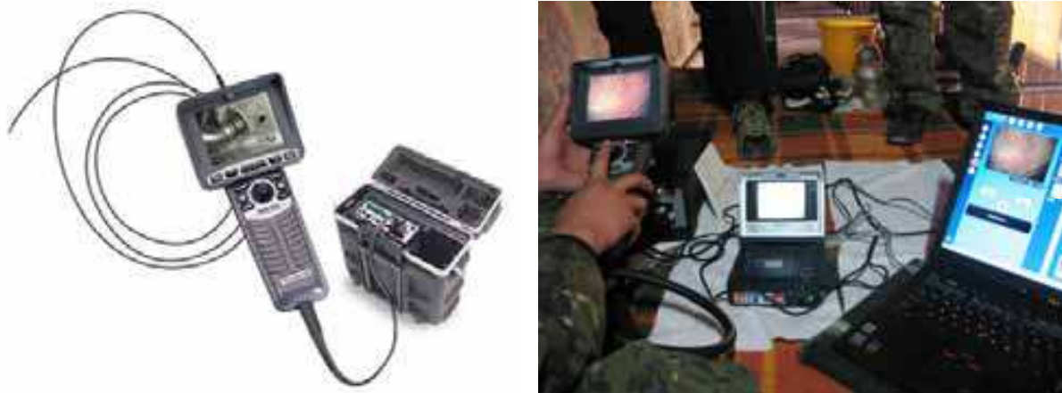
Fig. 15. XL PRO Video probe made by EverestVIT for remote visual test
