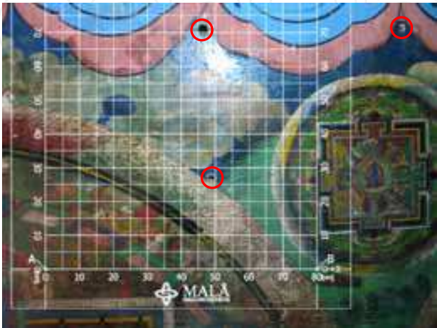
Fig. 17. Relative position of detection area to probing holes
