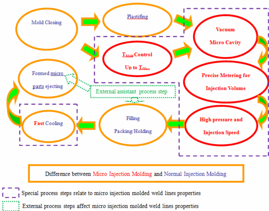
Fig. 1-2. Micro injection molding processing steps
