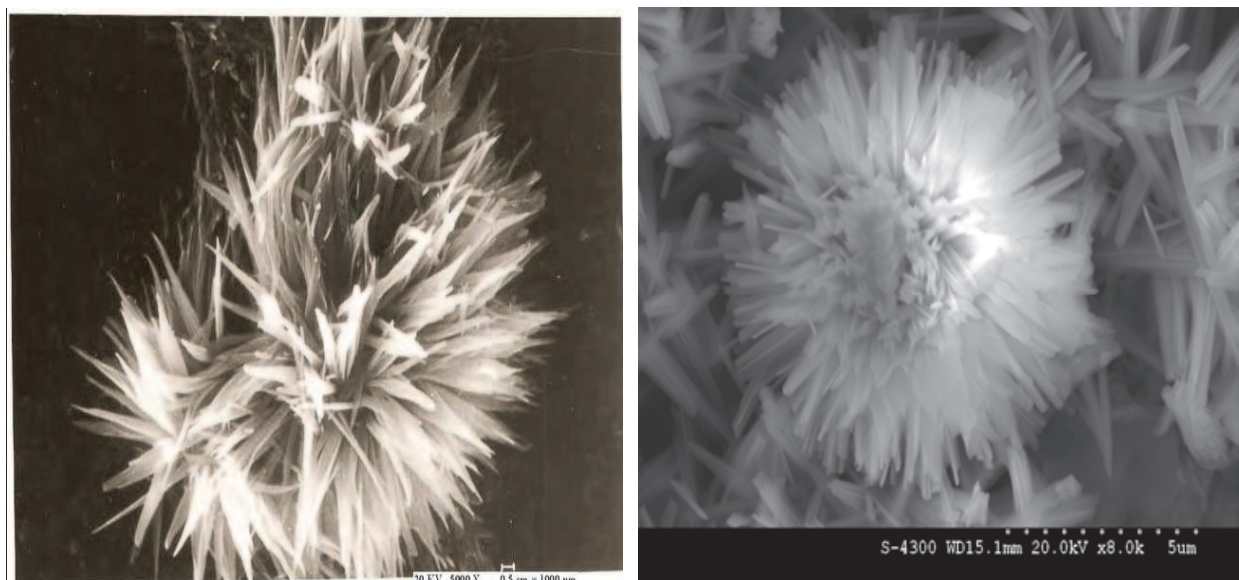
Fig. 5. FESEM micrographs showing flower patterns grown in polymer templates
