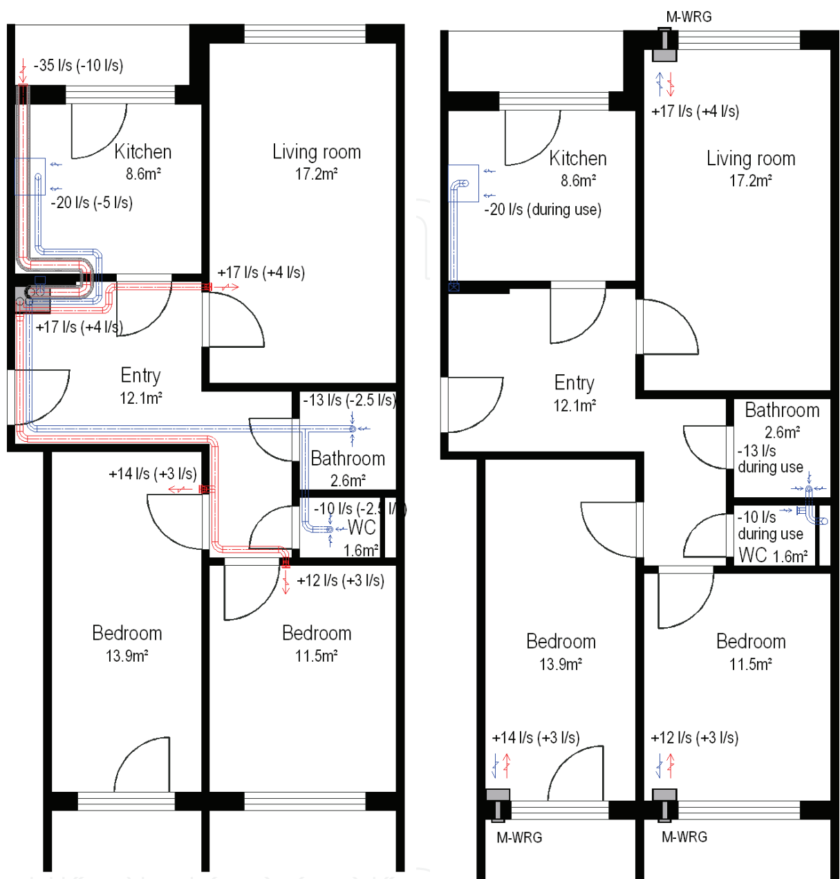
Fig. 16. Balanced ventilation solution with apartment AHU with heat recovery (left) and one room supply-exhaust AHU with heat recovery (right)
