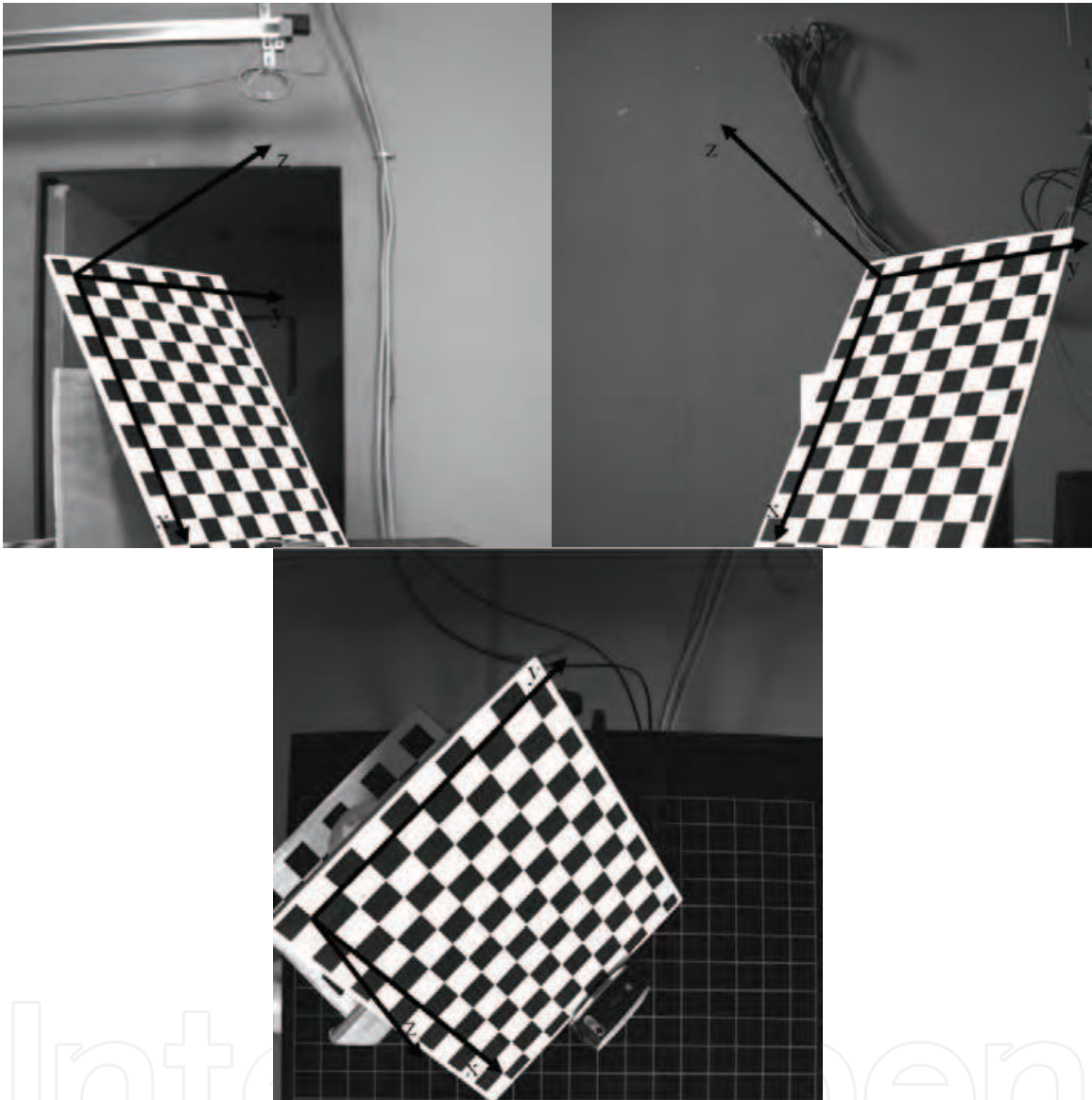
Fig. 4. The calibration target must be viewed simultaneously by all cameras when computing the common real world reference frame
