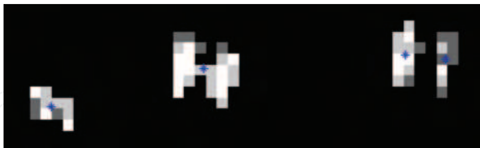
Fig. 10. Output of the center of mass calculation by weight averaging on three particles of the same image. Far left and center particles yield one centroid whereas far right particle displays two disconnected local maximum and therefore yields two centroids
