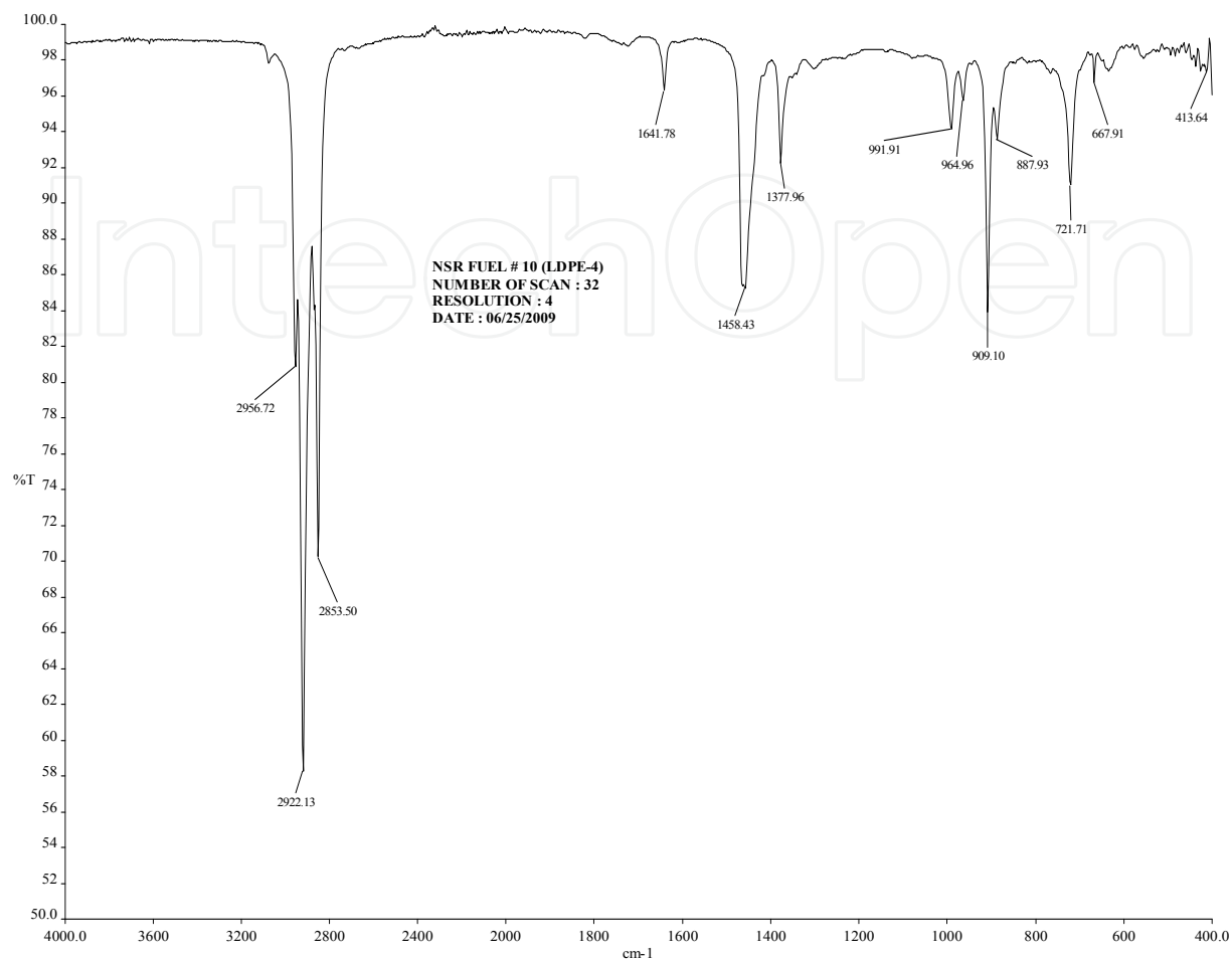
Fig. 17. FTIR Spectra of LDPE-4 Plastic to Fuel
