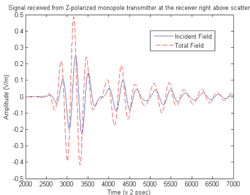
Fig. 6. Z-component of total and incident electric fields due to the monopole antenna, received at a receiver located right above the DNAPL pool.
