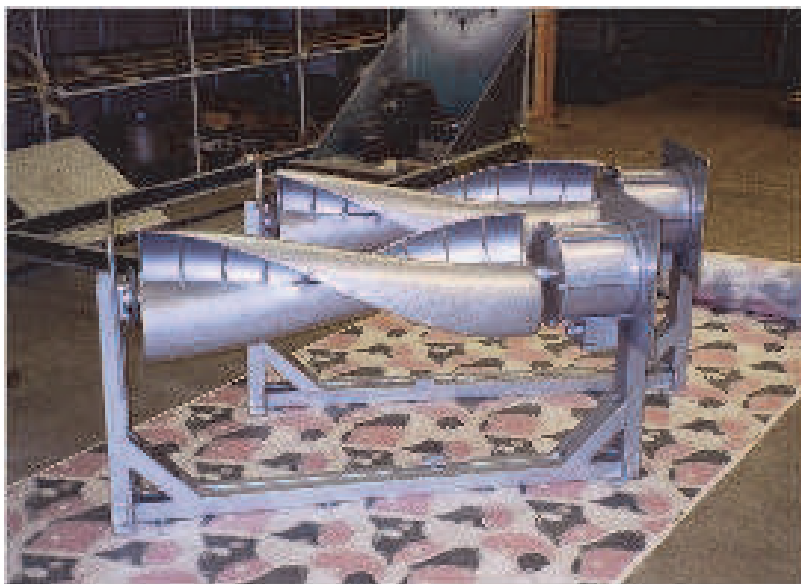
Fig. 5. Aesthetic VAWT made by Oy Windside in Finland
