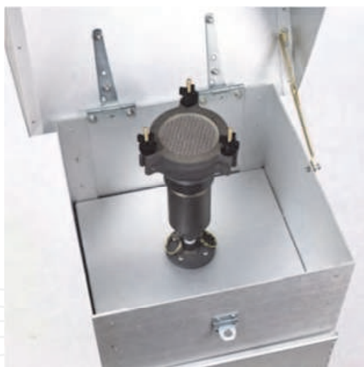
Fig. 2. Head of a PUF (polyurethane foam) sampler.
