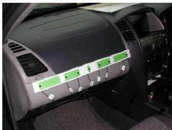
Fig. 8. A Microphone Array in Car
