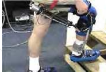
Figure 2. RoboKnee developed by Yobotics, Inc. ( RoboWalker , Dec. 2003)
