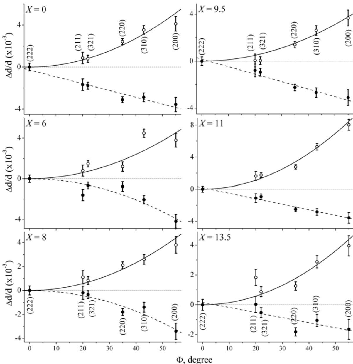
Fig. 8. Relative changes in the interplanar spacing  $\Delta d/d$ : longitudinal strains ( $\circ$ ), and transverse reductions ( $\bullet$ ) in the alloys with different silicon content  $X$  depending on the angle  $\Phi$  between the direction  $[hkl]$  and the closest axis  $\langle 111 \rangle$ . Lines show the variants of fitting by linear or quadratic functions of the angle.
