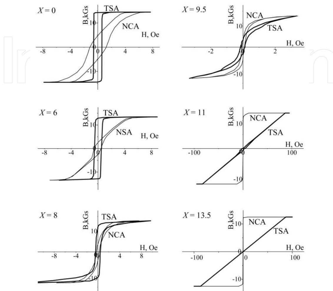
Fig. 1. Hysteresis loops measured for nanocrystalline  $\text{Fe}_{87-X}\text{Si}_X\text{B}_9\text{Nb}_3\text{Cu}_1$  alloy after the nanocrystallization annealing (NCA) and tensile stress annealing (TSA).
