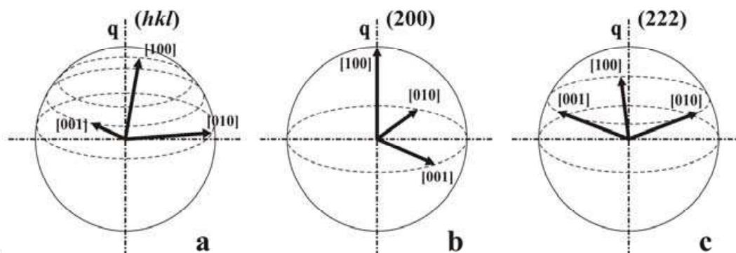
Fig. 10. Orientations of the axes of the nanocrystals contributing to the  $(hkl)$  reflection in the X-ray diffraction pattern measured during (a) the  $\theta$ - $2\theta$  scanning along the scattering vector  $\mathbf{q}$  and (b, c) special cases for the (b) (200) and (c) (222) reflections.
