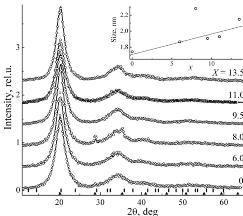
Fig. 3. Diffraction patterns of  $\text{Fe}_{87-X}\text{Cu}_1\text{Nb}_3\text{Si}_X\text{B}_9$  alloys in the initial state measured in the longitudinal (solid line) and transverse (circles) scans. The calculated positions of the peaks for the bcc structure of  $\alpha\text{-Fe(Si)}$  -  $\blacktriangle$ , and for  $\text{Fe}_3\text{Si}$  phase -  $\blacksquare$ . The inset shows the dependence of the average size of the regions with a short-range order on  $X$ .
