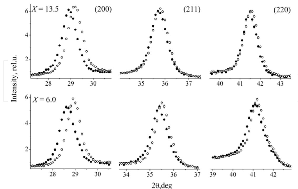
Fig. 6. Profiles of the diffraction peaks (200), (221) and (220) of the  $\text{Fe}_{87-x}\text{Si}_x\text{B}_9\text{Nb}_3\text{Cu}_1$  alloy samples at  $X = 13.5$  and 6 after TSA measured by scanning along (•) and perpendicular (○) to the ribbon or the direction of the load application during TSA.
