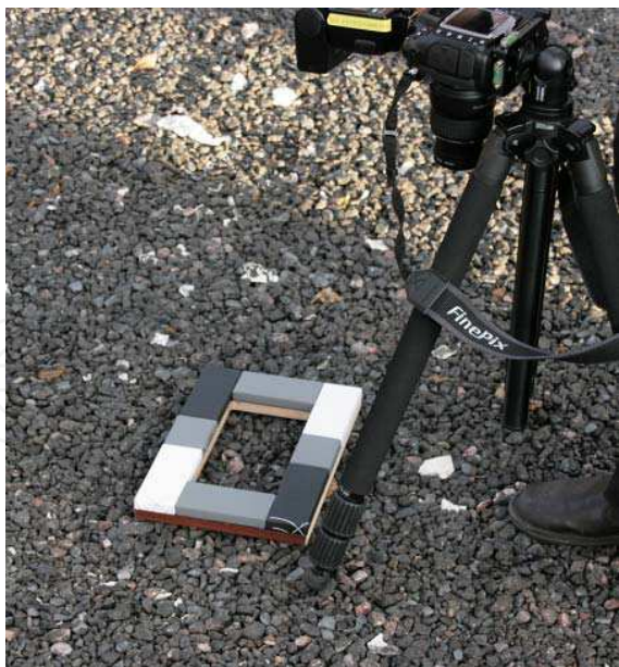
Fig. 6. Using digital camera and calibration frame to measure sample areas in Espoonlahti, Finland.
