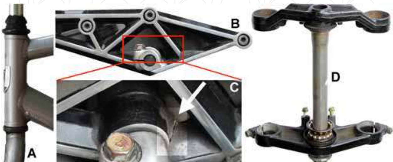
Fig. 1. Supporting structures in bicycle and motorbike engineering. (A) Headset of bicycle, (B),(C) subframe of motorbike with failure (arrow), (D) metal fork bridge of motorbike. © PBGF.
