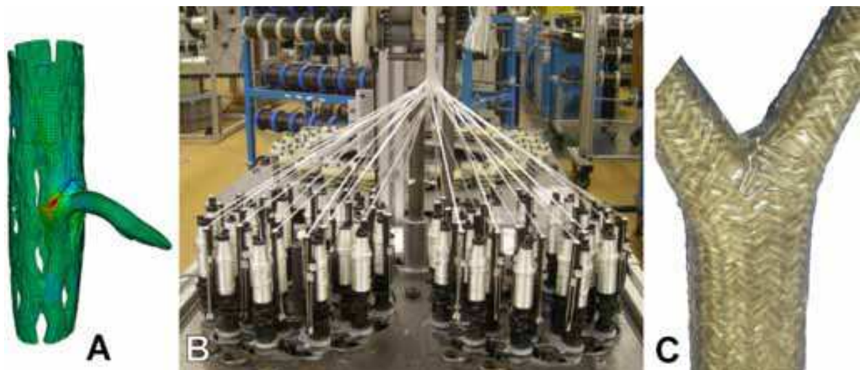
Fig. 28. (A) Simulated notch stresses in a stem-branch attachment region of a columnar cactus, (B) double braiding unit for producing branched braidings and (C) prototype of a braided Y-shaped preform. © (A) ILK Dresden, (B, C) ITV Denkendorf.
