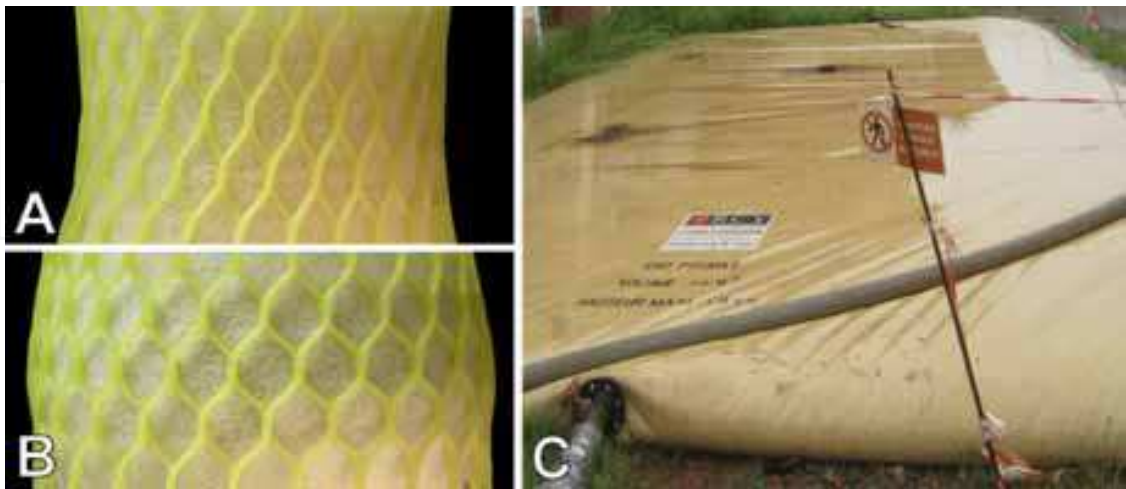
Fig. 23. Potential technical implementation for flexible hull structures. (A, B) Demonstrators combining a cellular matrix consisting of closed-cell foams and inextensible fibers, (A) undeformed state, (B) deformed state, (C) conventional flexible tank as an example for a potential technical application. © PBGF.
