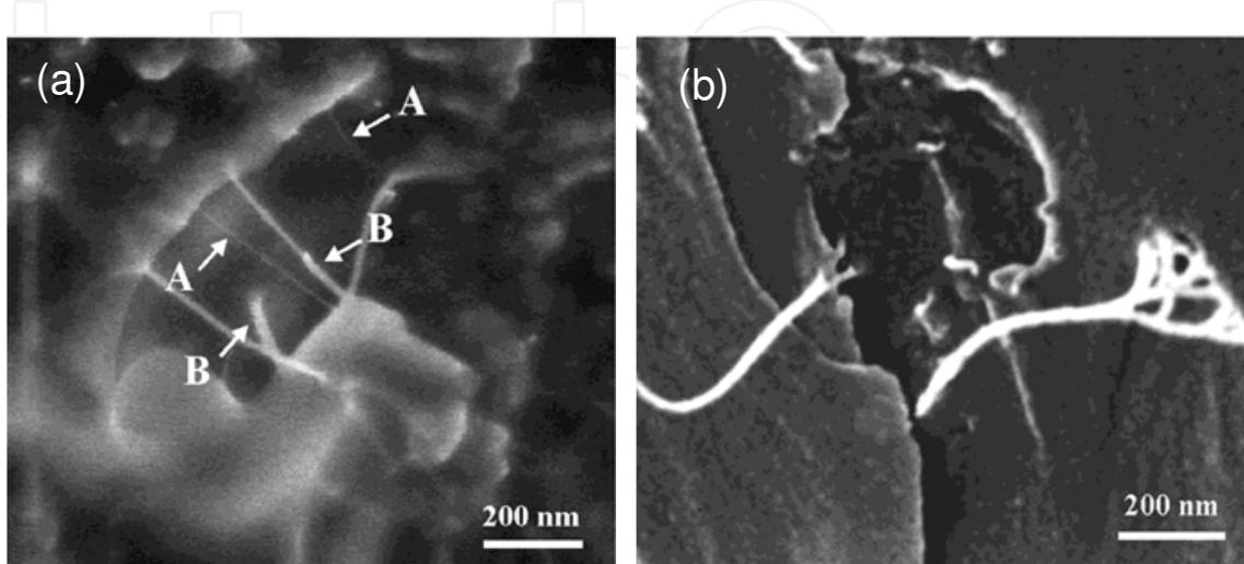
Fig. 24. Field emission SEM images of: (a) CNT-C<sub>16</sub>H<sub>32</sub>O<sub>2</sub>- epoxy composite for 0.8 wt % CNTs and 1:1 CNTs to C<sub>16</sub>H<sub>32</sub>O<sub>2</sub> weight ratio. The arrows indicate (A) individual CNTs and (B) CNTs covered with palmitic acid. (b) CNT-epoxy composite for 0.8 wt % CNTs without palmitic acid. The scale bar corresponds to 200 nm. Reproduced from Barrau et al., 2003a.
