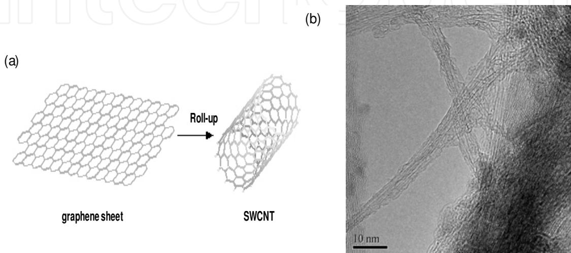
Fig. 3. (a) Formation of SWCNT. Reproduced with permission from [www.nanotech-now.com](http://www.nanotech-now.com) and (b) TEM image of SWCNTs.
