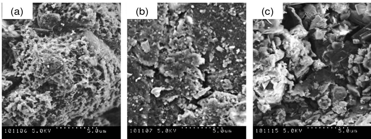
Fig. 13. SEM images for: (a) long-carbon nanotube-based CNT-200-EC electrode, (b) short-carbon nanotube-based CNT-2-EC electrode, and (c) conventional GEC electrode. Reproduced from Pumera et al., 2006.
