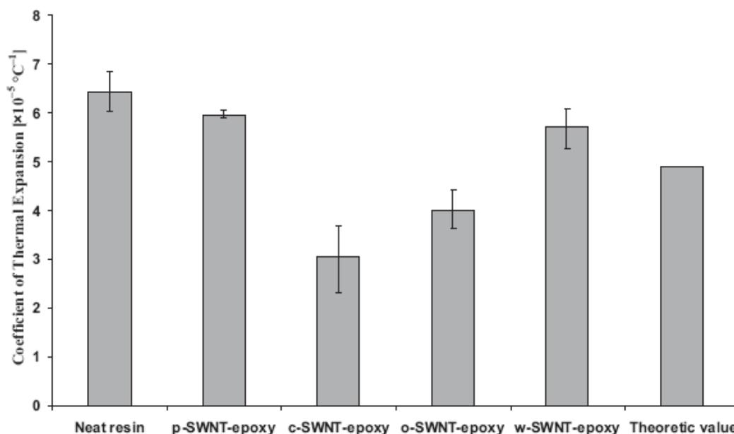
Fig. 30. CTE values of the neat epoxy resin and composites below the  $T_g$  range. Reproduced from Wang et al., 2007.
