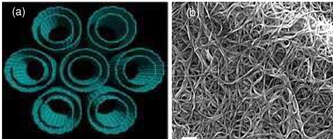
Fig. 5. (a) Computer generated image of DWCNT ([www.nanotechweb.org](http://www.nanotechweb.org)) and (b) SEM images of DWCNTs. Reproduced from Endo et al., 2005.
