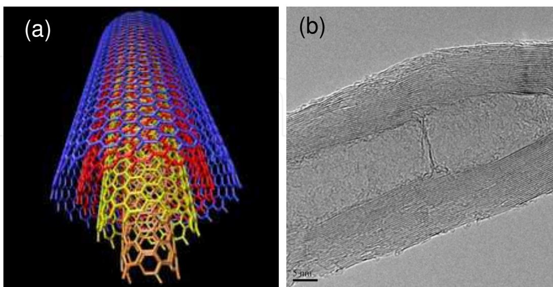
Fig. 4. (a) Computer generated MWCNT model. Reproduced with permission from [www.nanotech-now.com](http://www.nanotech-now.com) and (b) TEM image of MWCNTs.
