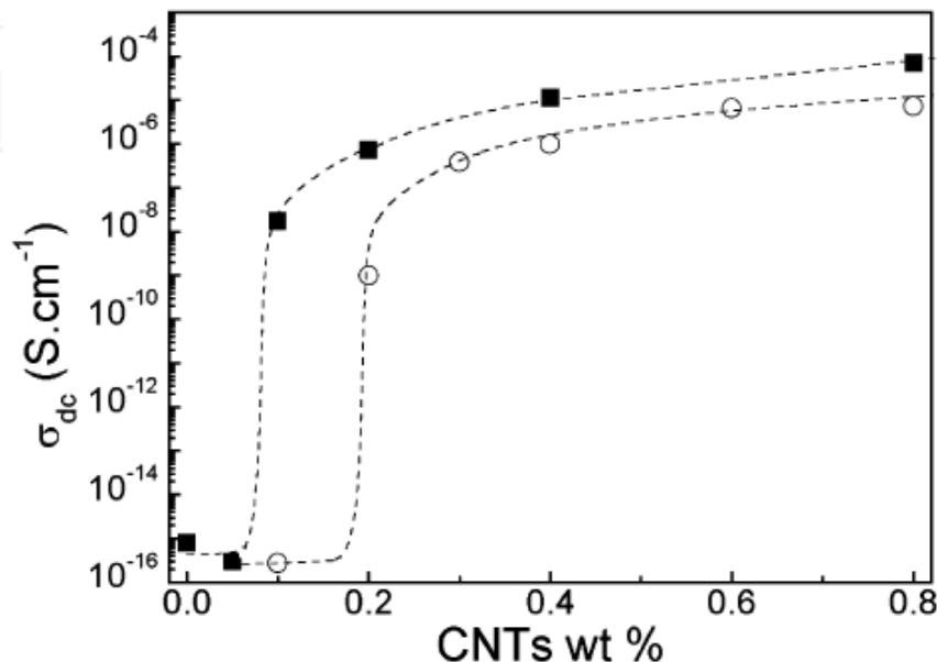
Fig. 31. Comparative plot of the dc conductivity dependence on the CNTs content at RT(■) with palmitic acid at 1:1 CNTs to  $C_{16}H_{32}O_2$  weight ratio and (○) without palmitic acid. Reproduced from Barrau et al., 2003a.
