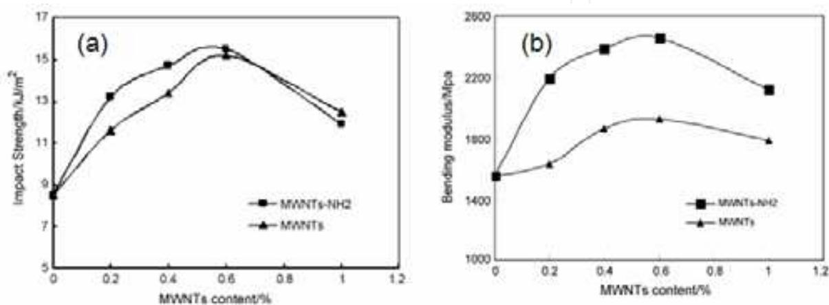
Fig. 17. The effect of MWCNTs and MWCNTs-NH<sub>2</sub> content on: (a) impact strength and (b) bending modulus of MWCNTs-containing epoxy composites. Reproduced from Yaping et al., 2006.
