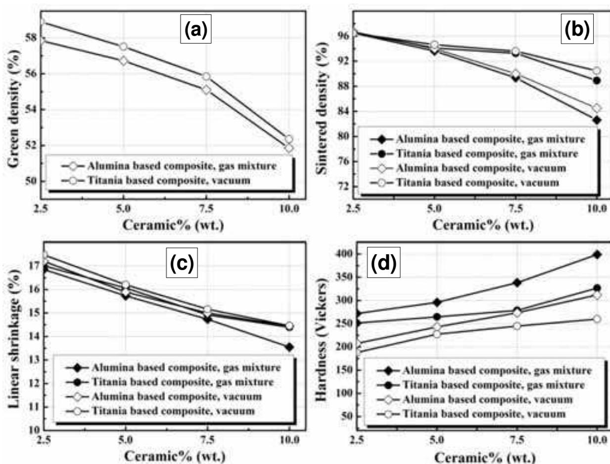
Fig. 4. Effect of ceramic inclusion on: (a) composite green density, (b) composite sintered density, (c) composite linear shrinkage and (d) composite Vickers hardness.
