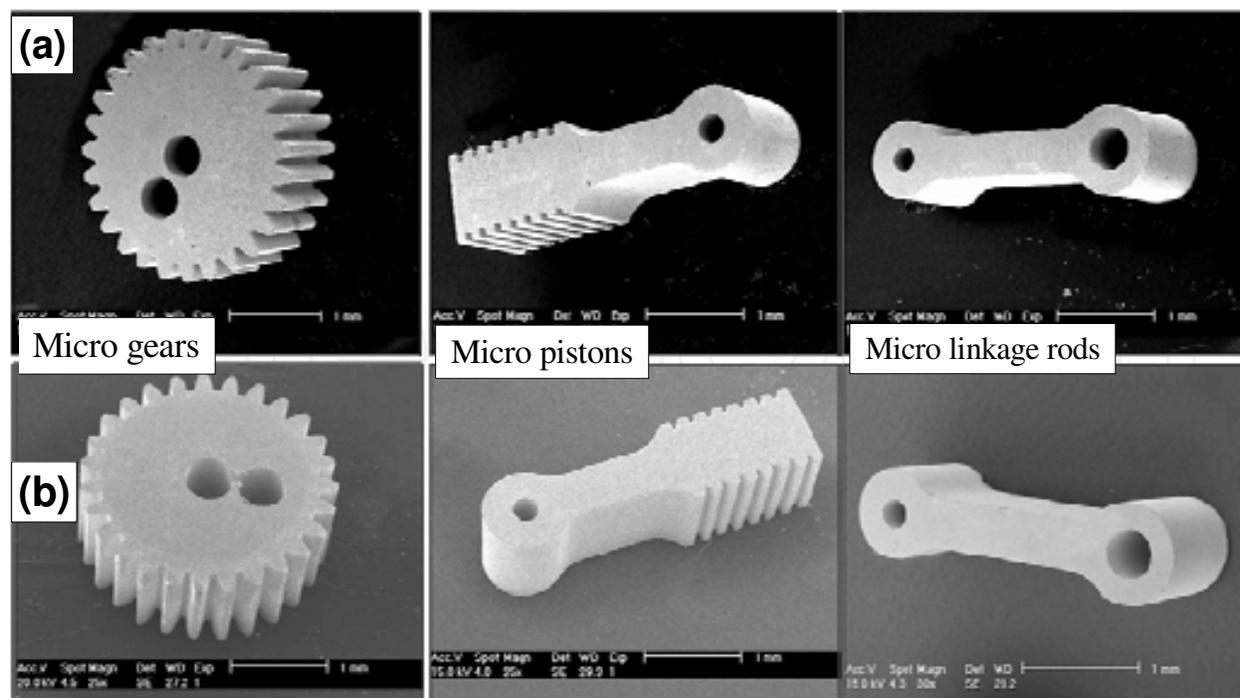
Fig. 2. SEM images of the composite green micro components based on: (a) 10% alumina and (b) 10% titania.
