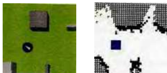
(a) Example of a robot environment with a robot inside it. (b) Incrementally constructed the histogram grid-based map.
