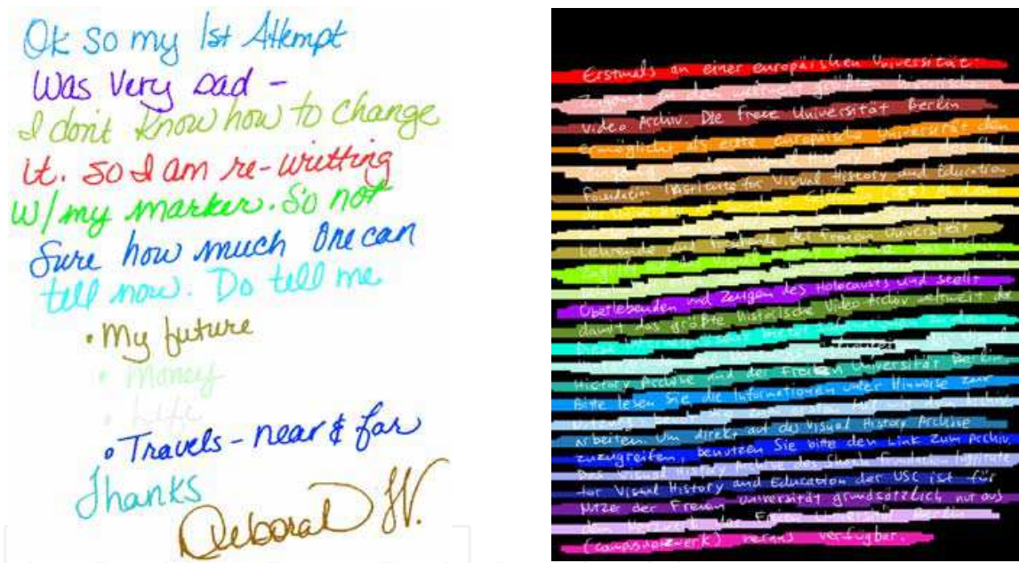
Fig. 2. Representation of text lines as: groups of text pixels with the same value (left) and parts of the document image (right)
