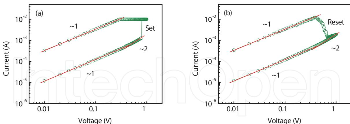
Fig. 6.  $I$ - $V$  curves of the the Cu/GO/Pt memory cell plotted in log-log scale and the linear fitting results in both LRS and HRS: (a) positive voltage region and (b) negative voltage region. Also shown are the corresponding slopes for different portions
