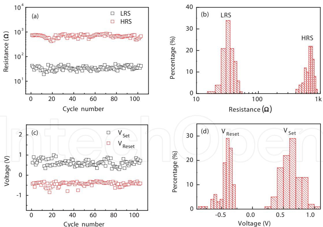
Fig. 4. (a) Endurance performance of the Cu/GO/Pt memory cell. The resistance values are read out at  $0.1$  V in each sweep. (b) Statistical distribution of the resistances in HRS and LRS. (c) Evolution of  $V_{\text{Set}}$  and  $V_{\text{Reset}}$  of the Cu/GO/Pt device as a function of the switching cycle. (d) Statistical distribution of  $V_{\text{Set}}$  and  $V_{\text{Reset}}$
