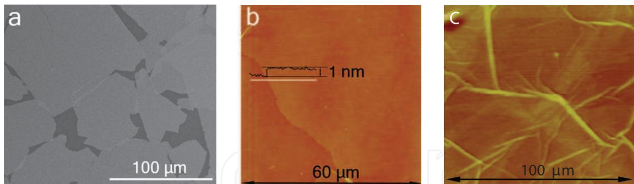
Fig. 2. (a) SEM and (b) AFM images of GO sheets that were deposited on a Si substrate by Langmuir-Blodgett assembly at a constant surface pressure of  $10 \text{ mN m}^{-1}$ . (c) AFM image of GO thin films of  $\sim 30 \text{ nm}$  in thickness prepared at room temperature by the vacuum filtration method
