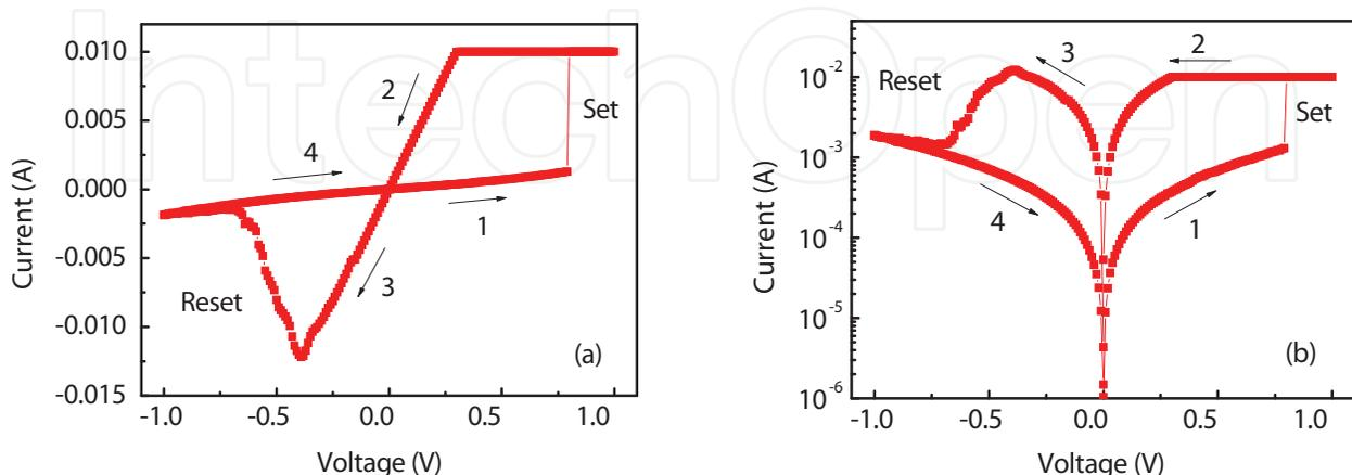
Fig. 3. Typical  $I$ - $V$  characteristics of the Cu/GO/Pt sandwiched structure shown in (a) linear scale, and (b) semilogarithmic scale. The voltage is swept in the direction as follows:  $0 \text{ V} \rightarrow 1 \text{ V} \rightarrow 0 \text{ V} \rightarrow -1 \text{ V} \rightarrow 0 \text{ V}$
