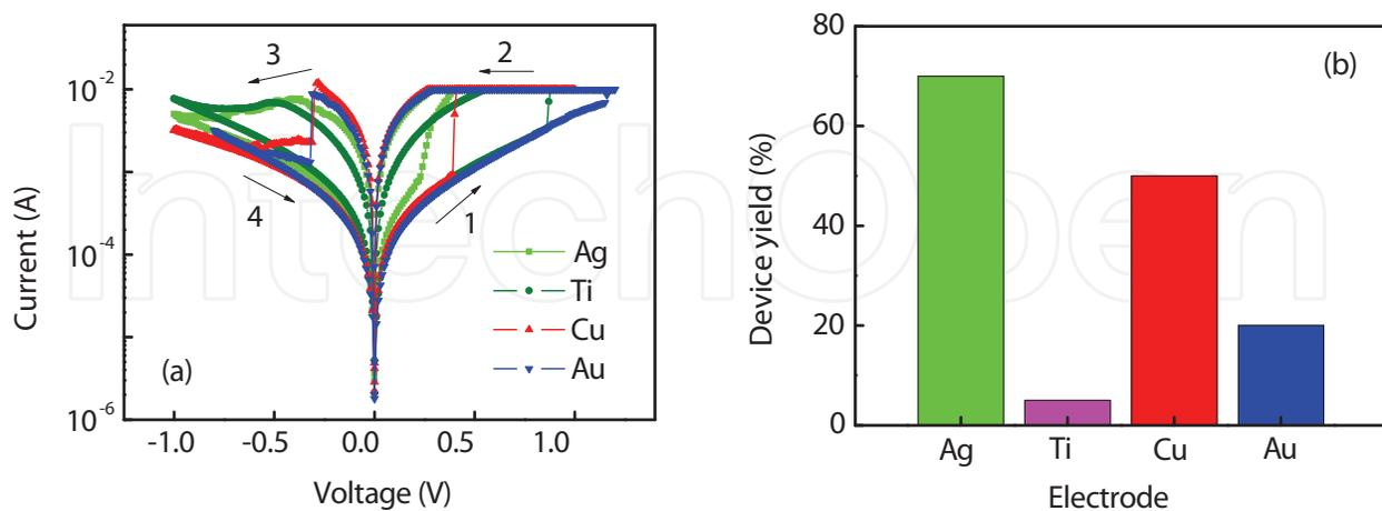
Fig. 8. (a) Typical  $I$ - $V$  characteristics of GO-based memory cells using different metals (Ag, Ti, Cu, and Au) as top electrodes shown in semilogarithmic scale. (b) Device yields of different metal/GO/Pt sandwiches
