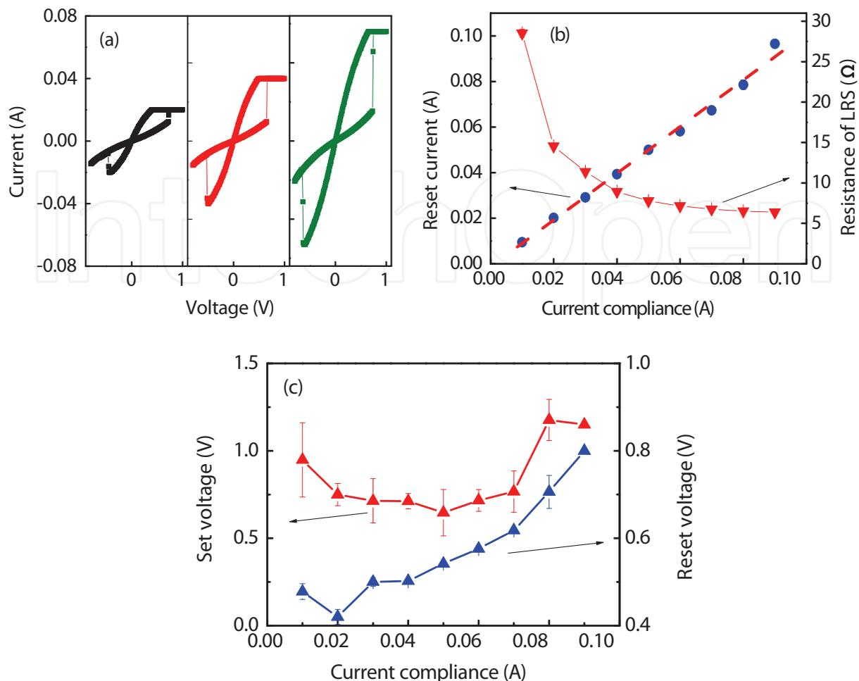
Fig. 12. (a) Typical  $I$ - $V$  characteristics of the Au/GO/Pt device with different current compliance (0.02 A, 0.04 A, and 0.07 A). (b) Current compliance dependence of the Reset current and resistance of the low resistance state of the Au/GO/Pt device. (c) Current compliance dependence of the Set and Reset voltages of the Au/GO/Pt device.
