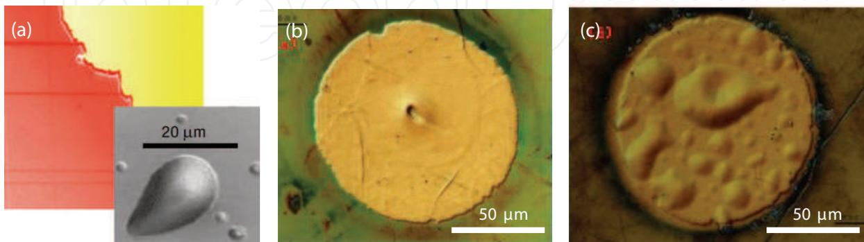
Fig. 11. Gas bubbles under the electrodes formed during the Forming processes of (a) the Pt/single crystalline SrTiO<sub>3</sub>/Pt memory cell (Szot et al., 2006), (b) Cu/GO/Pt memory cell with a GO thickness of 90 nm, and (c) Au/GO/Pt memory cell with a GO thickness of 30 nm
