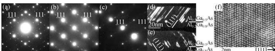
Fig. 9. Diffraction patterns of a twinned  $\text{Al}_{0.5}\text{Ga}_{0.5}\text{As}$  epilayer taking along (a)  $[110]$ , (b)  $[011]$ , and (c) nearly  $[011]$ . TEM images taking with a twin spot at (d)  $1/3, 1/3, 5/3$  and (e)  $\bar{1}/3, 1/3, 5/3$ . (f) A high-resolution TEM image of twin boundaries. (Ohno et al, 2007b)
