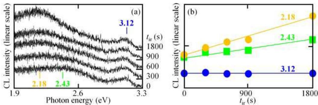
Fig. 6. (a) CL spectra after the irradiation of electrons, with flux of  $5 \times 10^{17} e \text{ mm}^{-2} \text{ s}^{-1}$  at temperature of 120 K, for the irradiation time  $t_{ir}$ . (b) The CL intensity at 3.12, 2.43, or 2.18 eV vs  $t_{ir}$ . (Ohno et al, 2009b). Copyright Wiley-VCH Verlag GmbH & Co. KGaA. Reproduced with permission
