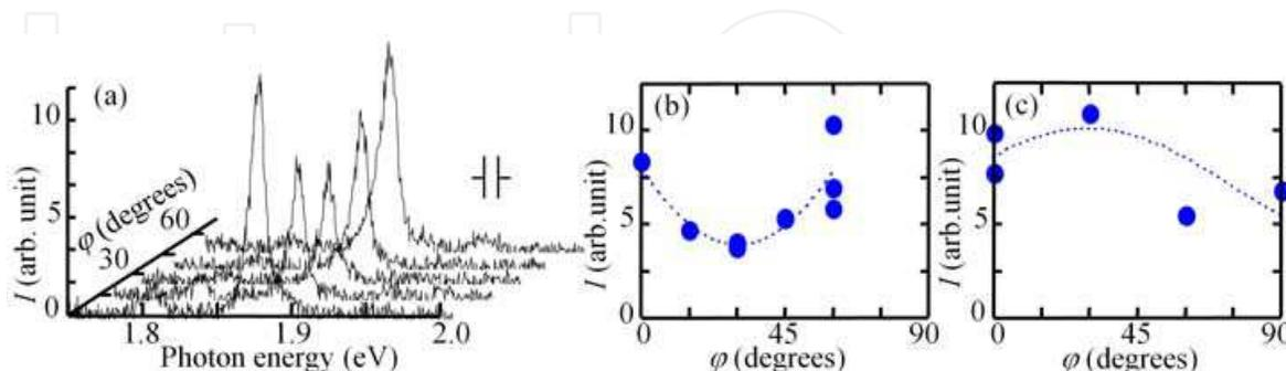
Fig. 12. (a) Polarized CL spectra for different  $\phi$  obtained from  $\alpha$  in Fig. 11b. The experimental setup is similar to that in Fig. 10a, and the specimen is set so that the  $z$  axis is parallel to [001]. The CL intensity  $I$  vs  $\phi$ ; the  $z$  axis is parallel to (b) [001] or (c) [110] (Ohno et al, 2007b)
