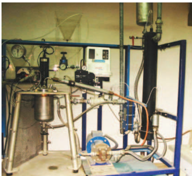
Fig. 2. The esterification reactor used for the experiments.
