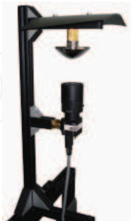
(b) Catadioptric imaging system
