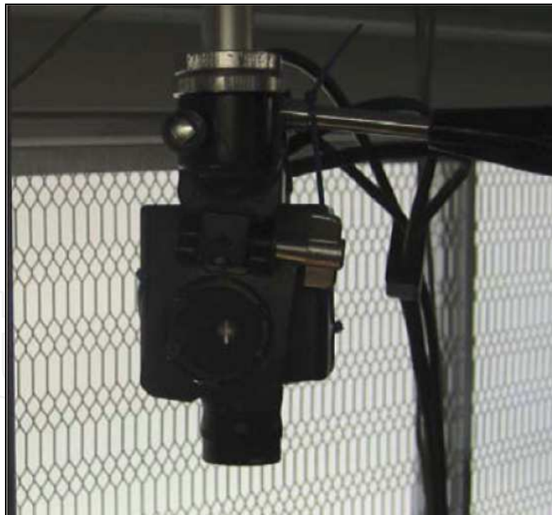
Fig. 11. Camera with image coordinate frame parallel to the robot coordinate frame.
