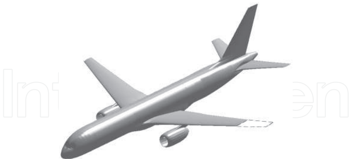
Fig. 2. Left Wing Damaged Generic Transport Model
