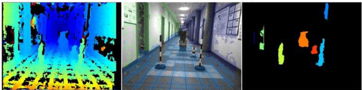
Fig. 4. The scene segmentation process: original depth map in pseudo-color (left), detection of planes overlaid on the original image (center), and grouping of objects which remain after removal of segmented surfaces (right)
