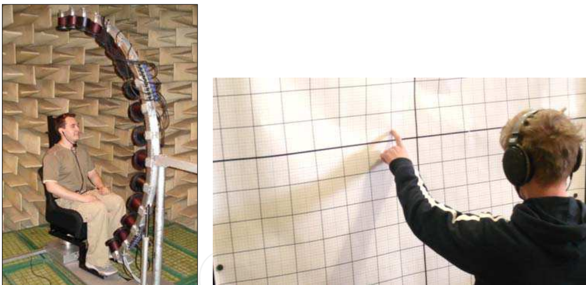
Fig. 7. The HRTF measurement setup in an anechoic chamber (left) and sound localization trials (right)
