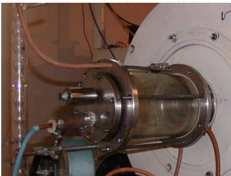
Fig. 5. Plasma chemical reactor with a volume of 6 litres
