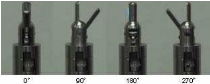
Fig. 9. Transition chart of the rotary gripper
