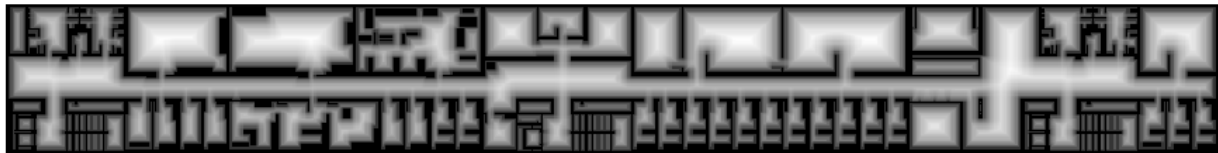
Fig. 10. Extended Voronoi transform of the UC3M Robotics Lab plan
