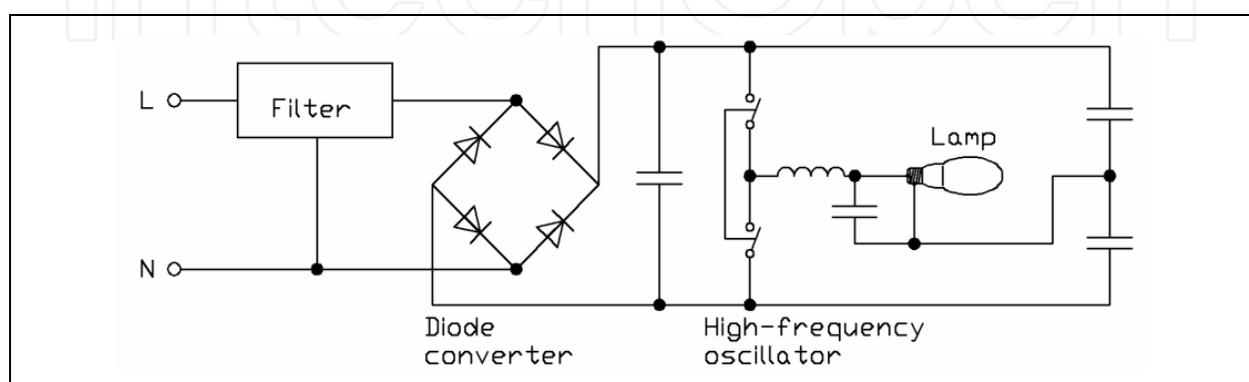
Fig. 4. Circuit diagram of an electronic ballast
