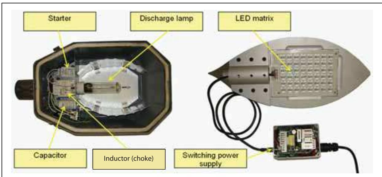
Fig. 1. Luminaire with discharge lamp and LED luminaire
