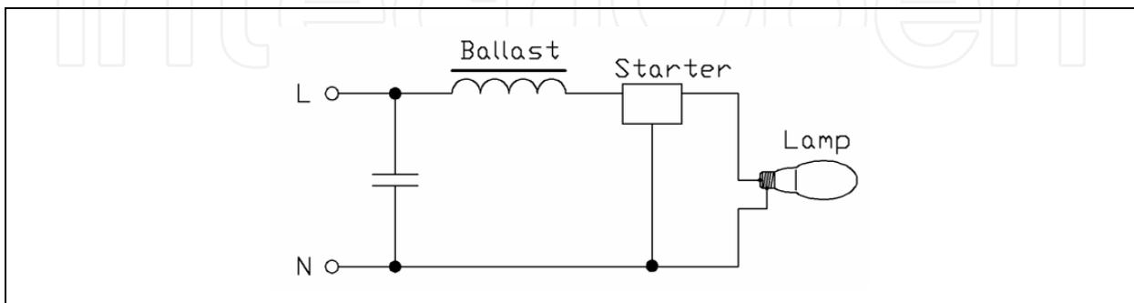
Fig. 5. Circuit diagram of a magnetic ballast
