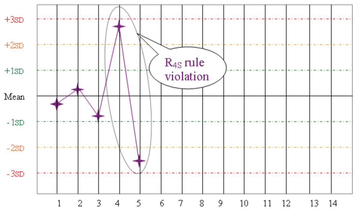
Fig. 5. Rule R_{4s} – when 1 control in a group exceeds the mean \pm 2s and another control exceeds the mean in the other direction by 2s, reject the run.
